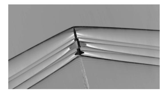
Schlieren image of supersonic aircraft with shock waves.
